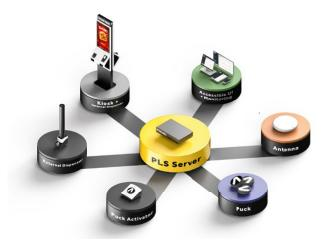
The heart of the PLS infrastructure is the hub. It receives data from the antennas and processes them using the most advanced algorithms. The hub provides a JSON API for seamless integration into your point-of-sale or pointof-service system.
