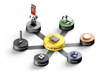
The heart of the PLS infrastructure is the hub. It receives data from the antennas and processes them using the most advanced algorithms. The hub provides a JSON API for seamless integration into your point-of-sale or point-of-service system.
